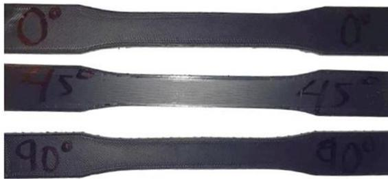
**Fig. 2.** ABS samples printed with printing angle of 0°, 45° and 90°
